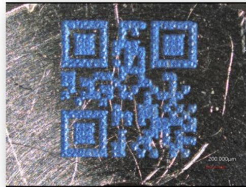
Fig. 1: UDI code obtained with the selective the titanium anodization process
