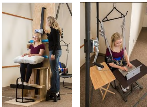
Fig. 1: Left: Spinal height stadiometry measurement; Right: subject testing in vertical traction harness.
