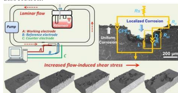
Fig.1: Schematic of the vascular bioreactor with an electrochemical monitoring system. Equivalent electrical circuit used to fit the EIS data shown on the cross-section of the corroded sample at each FISS and time condition. Typical 3-D reconstructions using X-ray micro-CT of samples with the increase of FISS.
