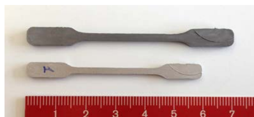
Fig. 2: Green (top) and sintered (bottom) parts.
