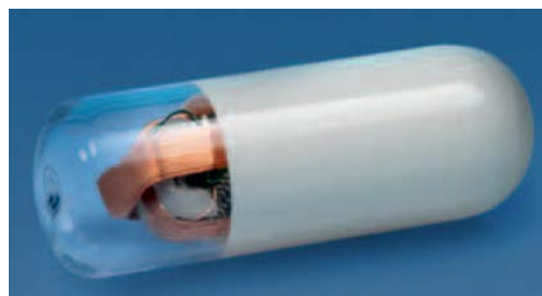
Fig. 2: Images of a Cylindrical Glass Encapsulation for diagnosis of the digestive system (Motilis Medica, D: 8.25mm; L: 25 mm).
