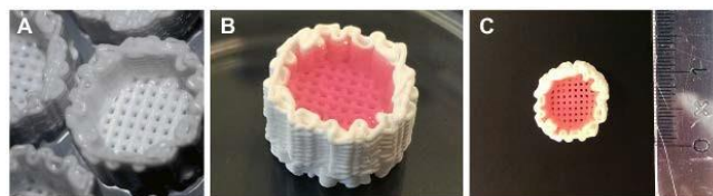
Fig. 2: 3D printed ceramic scaffolds (A), which can be functionalized with osteogenic differentiated MSCs, acting as a bone-like compartment to the soft bone marrow culture (in pink, B, C.)
