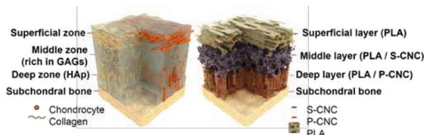
Fig. 1: Schematic representation of the architecture of native hyaline cartilage (left) and the multi-zonal scaffold (right). Reprinted from Camarero-Espinosa, S. et al. Biomaterials 74, 42-52 ©2016.
