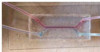
Fig. 1: Microfluidic device with coloured liquid in the channels.
