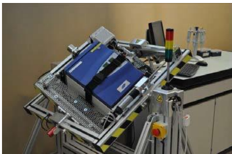
Fig. 1: Random Positioning Machines (RPM) are used as a ground based model for simulated microgravity.
