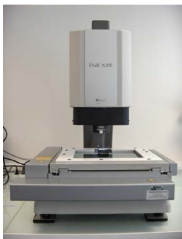
Fig.1 : Evaluation of the dimensional reliability with the video measuring system Nikon® Inexiv
