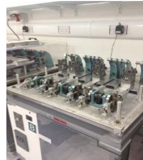
Fig. 1: Six station pin on plate friction rig, for nano-scale wear debris generation.
