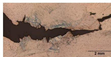
Fig. 2: Crack propagation and twinned grains.
