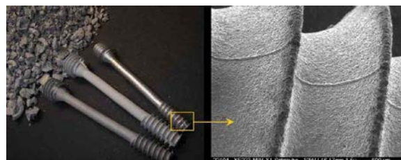
Fig. 2: Green-, debinded- and sintered MIM-part of an implant prototype bone screw made of Mg X1 alloy
