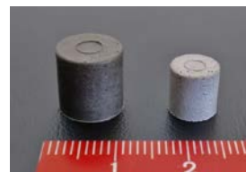
Fig. 2: Green and sintered porous titanium parts.
