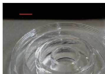
Figure 2: 3D printed construct with PF127. The red bar indicates 2 mm
