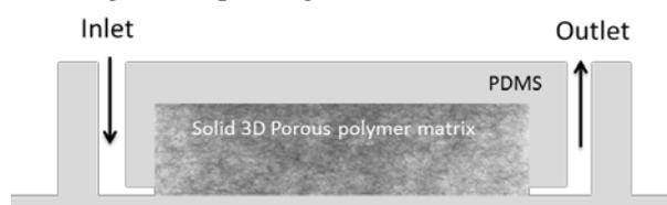
Fig. 1: Schematic cross-section of the microfluidic device
