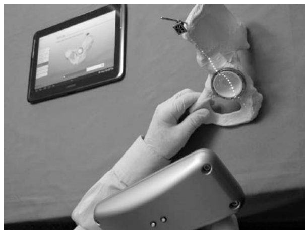
Fig. 2: The laser scanner of the system measures the surface of a hip joint prosthesis inserted into a pelvis model.
