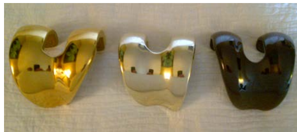
Fig. 1: left: PVD-Medthin™ 01 TiN. TiN is FDA approved since 2002 and sold in USA, Europe, Australia and emergent markets, etc; middle: PVD multilayer Ionbond-Aesculap AS coating 510K approved, on sale in USA, Europe and other countries; right: CVD dual and multilayers coatings by Ionbond.
