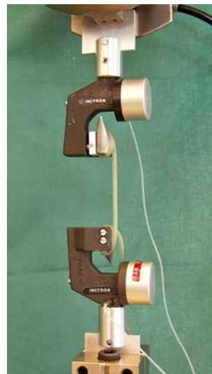
Fig. 1: Set-up for tensile testing of feeding tubes. Photo: NR Gjerdet.
