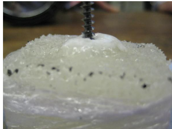
Fig. 1: A 4mm screw in cancellous bone substitute augmented with HydroSet® showing the displaced dome of cement.
