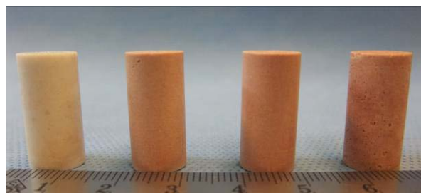
Fig 1: PMMA samples with increasing amount of bone marrow. Left to right: 0.0, 2.5, 5.0, 7.5 ml.
