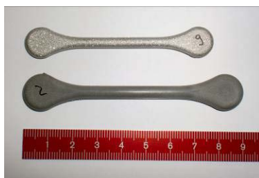
Fig. 2: Injection moulded and sintered Ti-17%Nb MIM test specimens
