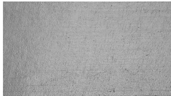
Fig. 2: Surface finish of the same TiAl6Nb7 screw as in Fig. 1 after rework by CET processing, Ra = 0.07 µm. Mag. 700 x
