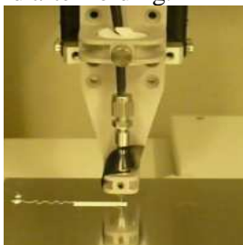
Fig. 1: robotic deposition of UV curable pastes.
