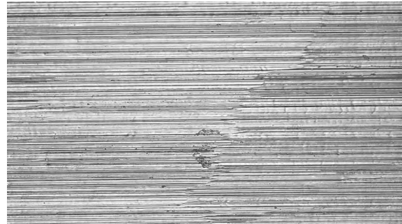
Fig. 1: Surface finish and roughness in the groove of threads of a TiAl6Nb7 screw processed by thread whirling, Ra = 0.2 µm. Mag. 700 x
