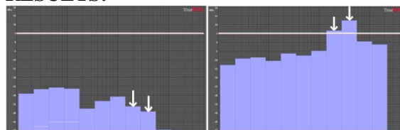
Fig. 1: Frequency profile of a paste prior to setting (left) vs. immediately on setting (right).
