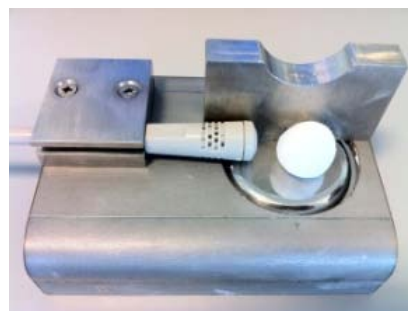
Fig.2: Apparatus used containing microphone, plate and sample drop height guide.
