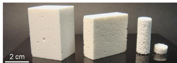
Fig. 1: Ceramic scaffolds with different microstructures machined into the desired shapes.
