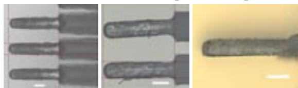
Fig. 1: Injection molded 100 \mu\text{m} -wide COC (left), POM (center) and PP (right) cantilevers. Scale bars 100 \mu\text{m}
