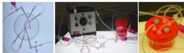
Figure 1: Closed loop bioreactor system. Preliminary co-culture experiments have also begun to investigate the effect of glial-neuronal cultures on different surface chemistries.
