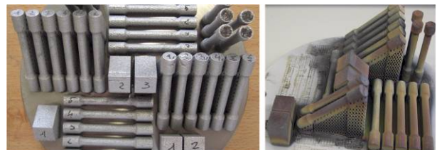
Fig. 2: Left: Native SLM processed tensile probes. Right: Probes after heat treatment in argon atmosphere at 925°C for 4 hours.
