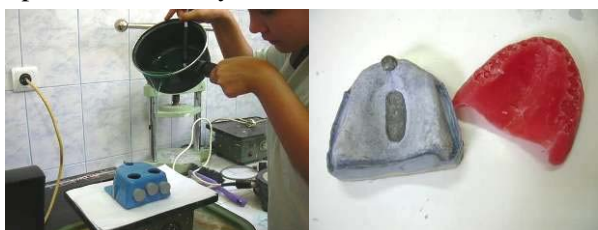
Fig. 1: The wrapping of the final pattern (left), pattern resulting after the removal of the denture base pattern. (right).
