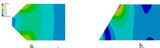
Fig. 1: Presentation on the longitudinal section of welded plates for the stress areas according to the welding type: a. on two faces; b. on one face
