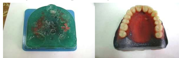
Fig. 3: Bubbles in the reversible hydrocolloid (left), melting of the wax pattern (right).
