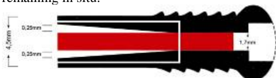
Fig 1: The design of the implants to test crevice and/or galvanic corrosion.
