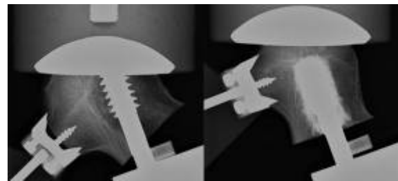
Fig. 3: Typical appearance of a cut-out after mechanical testing. The augmented specimen went through the entire testing protocol (3.0 cc of PMMA cement around screw).
