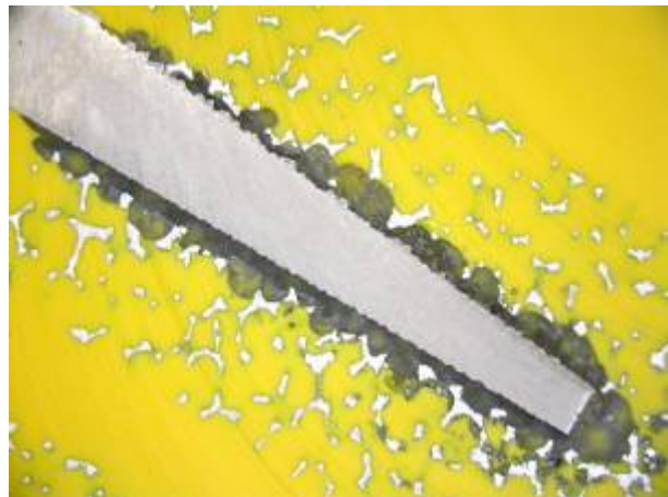
Fig. 2: Hybrid implant inserted into low density aluminium foam (substitute material for osteoporotic bone)
