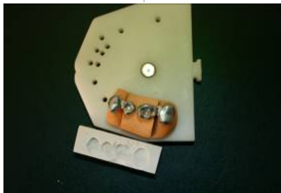
Fig. 3. The Titanium bridge after welding.
