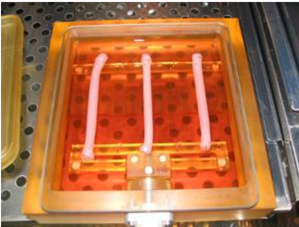
Fig 1: Three tendon constructs after transfer into the bioreactor for cyclic stretching.
