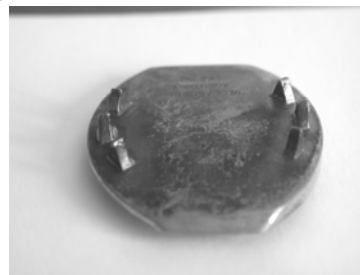
Fig. 1: Charite disk bearing a covalently linked layer of collagen.. Toluidine blue staining shows coating homogeneity
