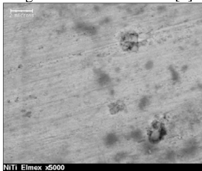
Fig. 5. SEM photomicrograph x 5000 of NiTi after oxidation in Elmex® solution
