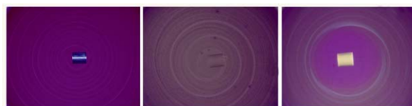
Figure 1. Growth inhibition of S. epidermidis ATCC 35989 on agar plates. A) titanium, B) poly(lactide-co-glycolide) (PLGA) 80/20, C) PLGA 80/20 containing ciprofloxacin.
