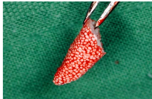
Figure 1: \beta -TCP/PLGA open porous copy of the root of a mandibular third incisor of a mini-pig. The open porosity of the scaffold allows the absorption of autologous blood.
