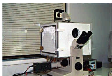
Fig 1: Inverse phase-contrast-microscope equipped with a styrofoam isolated lucite cube to maintain hemostasis over a longer period.
