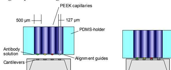
*Fig.3: Four PEEK capillaries embedded in a PDMS holder are used to deposit the solutions.*
