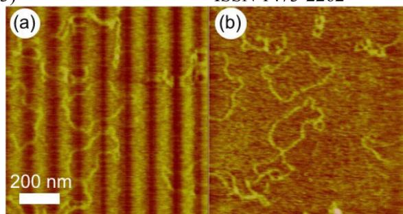
Fig. 2: Topography of pUC-18 plasmid DNA imaged at 61Hz line-scan rate. (a) Standard PI controlled system and (b) model-based controlled AFM. Images are recorded from right to left. Height scale: 3 nm.
