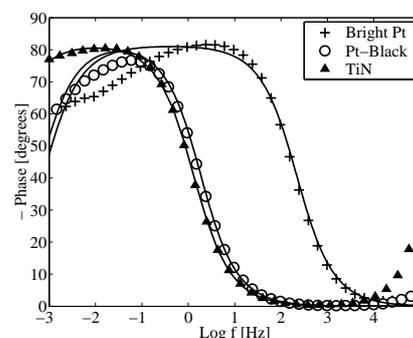
Fig. 3: Phase experimental results for the  $1 \text{ cm}^2$  bright Pt, Pt-black and TiN electrodes. Modeled results given by solid lines.
