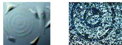
Fig.4. Micro structuring of PEO surfaces. Lithography processes were used to generate patterns of various surfaces preventing or facilitating cell adhesion.
