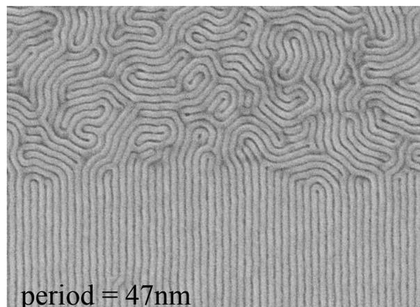
*Fig. 1: Epitaxial self-assembly of a block copolymer film on a surface patterned with X-ray interference lithography. The upper part of the SEM image shows the random orientation of the block copolymer domains in the un-patterned area of the sample whereas the domains in the lower part have aligned themselves to the lithographically defined surface template.*
