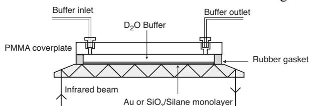
Fig. 1: Flow cell featuring a transparent polymethylmethacrylate coverplate which is pressed against a thin perfluorinated elastomer gasket to form a watertight seal. A computer-controlled piston pump enables rapid and efficient exchange of the buffer.
