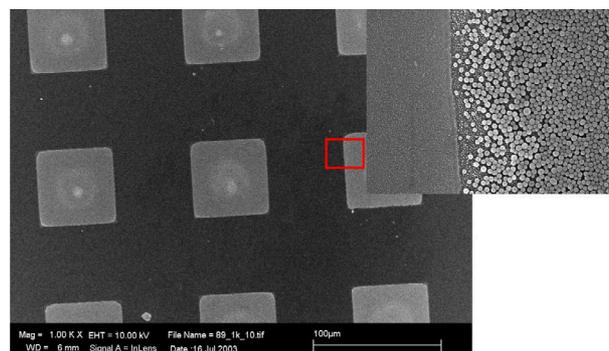
*Fig. 1: SEM image of 60µm squares ( $\text{SiO}_2$ ) covered with self-assembled  $\text{SiO}_2$  particles (35nm). The  $\text{TiO}_2$  background is modified with a hydrophobic alkane phosphate SAM and is particle free due to de-wetting during drying.*
