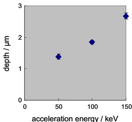
Fig. 1: Depth of the grooves fabricated on biodegradable polymer by ion beam irradiation.
