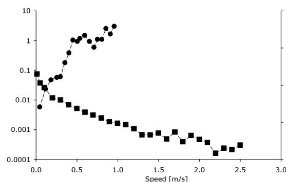
Fig. 2: A direct comparison of the coefficient of friction (y-axis on the left side) and the lubricant film thickness (y-axis on the right side).
