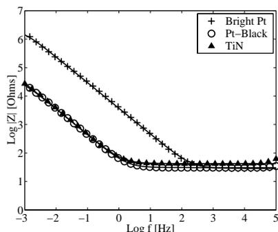
Fig. 2: Impedance modulus experimental results for  $1 \text{ cm}^2$  bright Pt, Pt-black and TiN electrodes. Modeled results given by solid lines.
