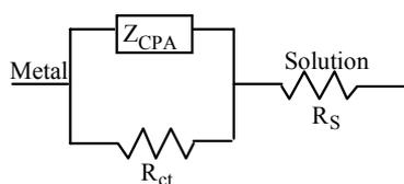
Fig. 1: Equivalent circuit model.
