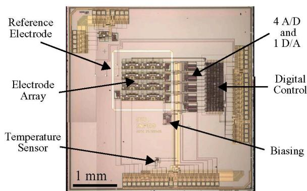
Fig. 1: Micrograph of CMOS Chip with main components.
