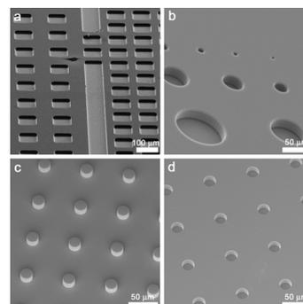
*Fig. 1: SEM micrographs of a) wet-etched structures in glass; b) ICP-etched Si-Master; c) replicated PDMS structures; d) hot-embossed structures in PS. (scale: a: 100  $\mu\text{m}$ , b,c,d: 50  $\mu\text{m}$ )*
