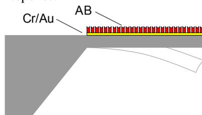
*Fig. 1: A silicon cantilever with a single-side antibody coating for static measurements. When analyte molecules attach to the antibody layer, the resulting surface stress bends the cantilever.*
