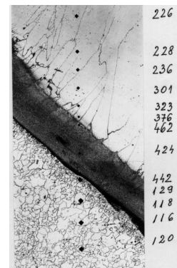
Fig. 1: Micrograph of zones and layering in a typical heterogeneous sample (metallurgical).
