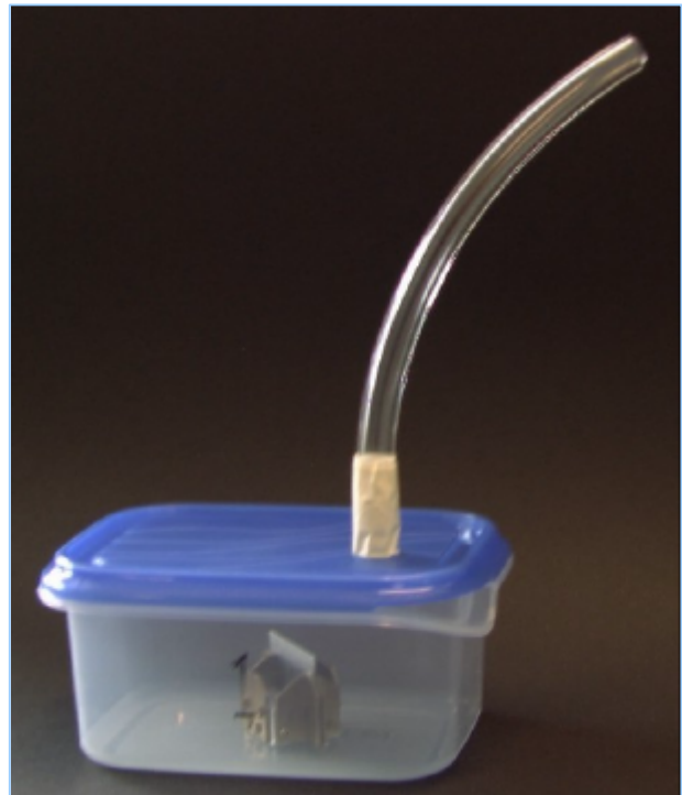
Fig. 2: Warming-up device used to bring cold fractured articular cartilage samples back to room temperature.
