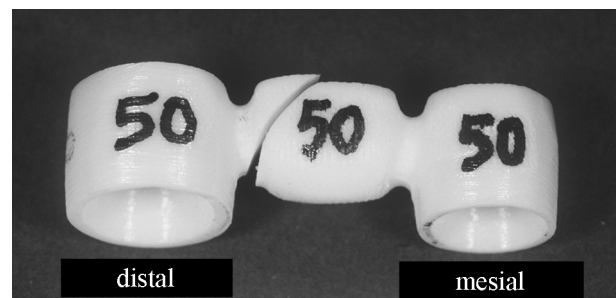
Fig. 3: Fracture of a framework in the connector.
